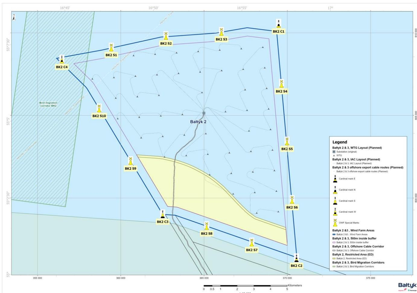
Figure 3 – Layout of demarcation buoys in Bałtyk 2 OWF
