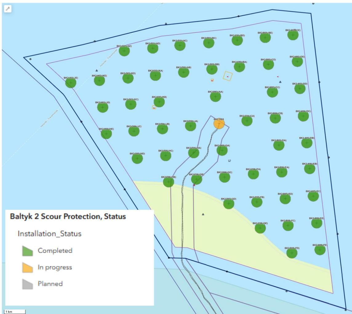
Figure 4 – Bałtyk 2 OWF Scour Protection Installation Overview (20.02.2026)
