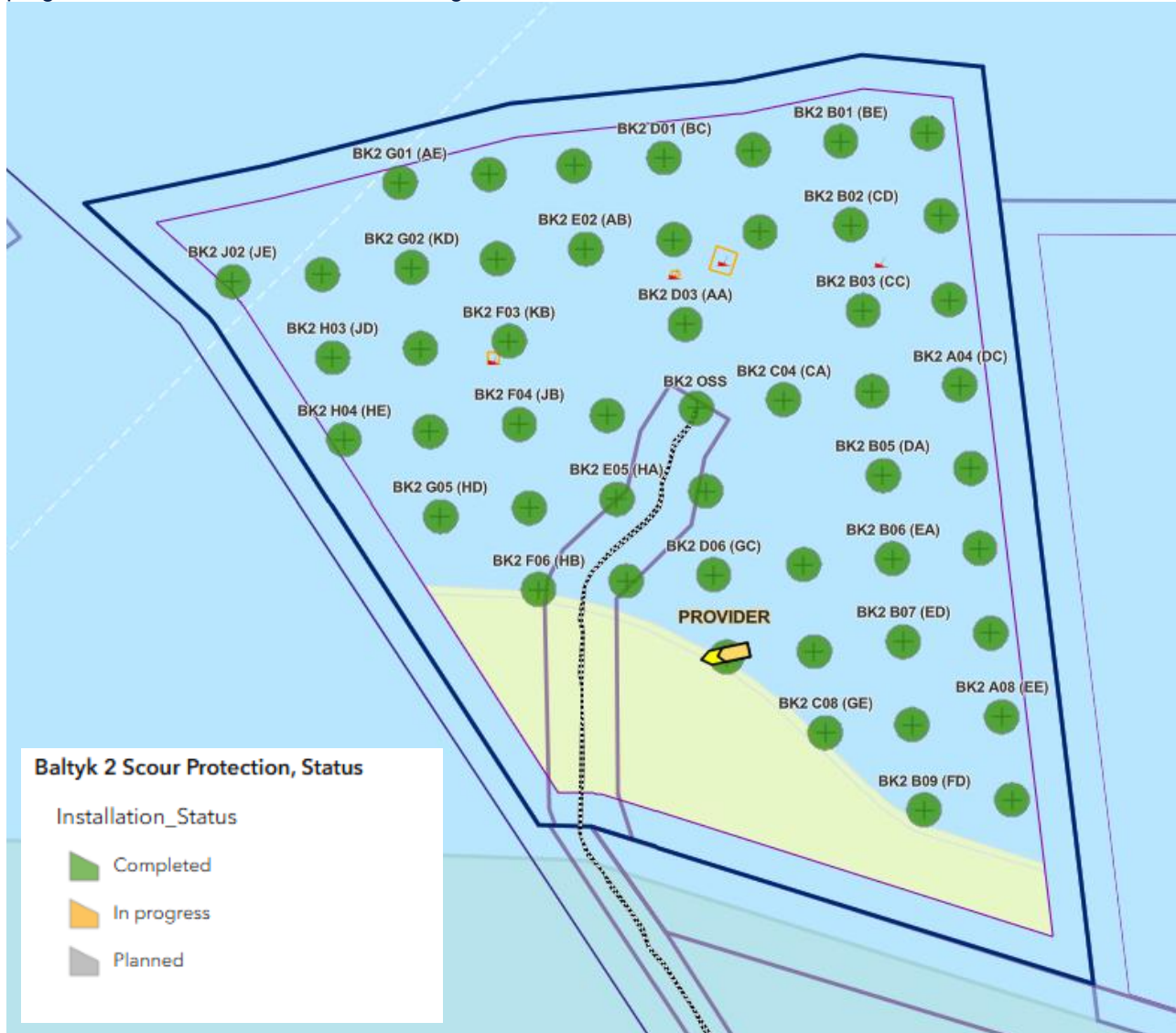
Figure 5 – Bałtyk 2 OWF Scour Protection Installation Overview
