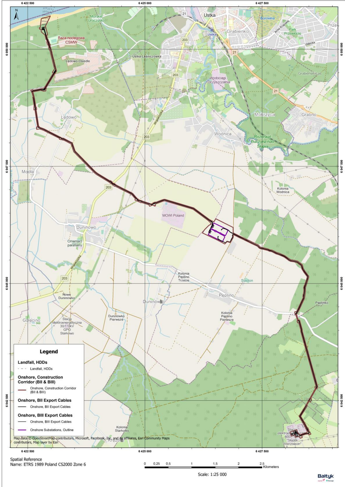
Figure 3 Onshore connection infrastructure of the MFW Bałyk II and MFW Bałyk III
